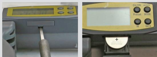
When the battery is removed, the battery may stuck in the housing. In this case, press the battery cover down slightly and pull it out.
