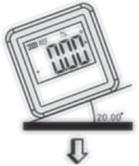
Put the instrument on the surface that needs to be measured, or change the angle on the reference surface, the readout displays the angle value relative to the reference surface (here it is 25°).
