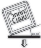
Short press the ABS/REF button to change to relative measuring mode. The display is set to "0.00 °" and "R" appears. Press it again to change to absolute mode.
